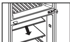
Gently hold the shelf provided in Freezer/Refrigerator compartment from the front side properly. Tilt it slightly from the front side to down and take out the shelf slowly.
