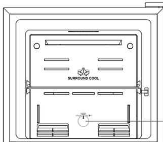
The airflow control in the freezer, control the distribution of cold air between the refrigerator compartment & freezer compartment, turn knob to the left for Normal ice to the right fast Ice setting, As per recommendation, it should be present in the Normal position for uniform cooling in freezer and refrigerator compartment.
