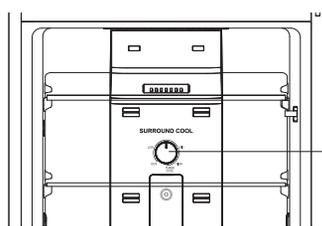
To control the temperature of refrigerator, turn the knob according to your requirement. This control is provided inside the refrigerator section. Turn knob to the left side to reduce the cooling and turn to the right to increase the cooling.
