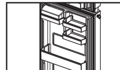
Gently hold the Door Bins provided in Refrigerator and freezer compartment from the side walls. Now lift the Door bin towards upward direction until it is out of its holding area.
